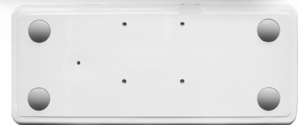
300XXX00 bottom: 6 rubber feet, 4 x 5mm, 2 x 15mm supplied for different angles + Brass inserts on 75 mm VESA distance
